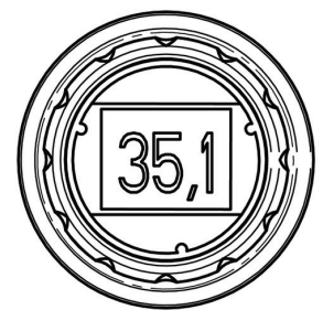
Panel mounting Ø110 mm front flange with 3 x Ø4 mm holes for screws
