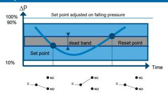
A flexible sensing element actuates a microswitch by means of a piston. The set point is adjusted by means of a compressible spring installed in opposition.
