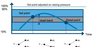
Set point and reset point must be between 10% and 90% of the selected scale.
