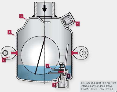
internal parts of deep drawn CrNiMo stainless steel (316L) long operational lifespan
