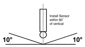
Figure 2. Dimensional Drawing for the Rosemount 3900/3900VP Sensor
