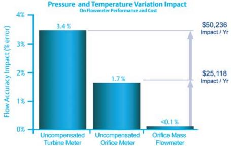
\* Pressure variations due to flow through 100ft (30m) of 4" (100mm) pipe with 4 elbows
