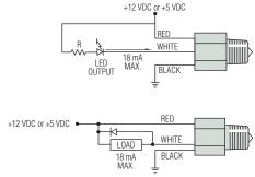
Note: Inductive loads must be diode suppressed.
